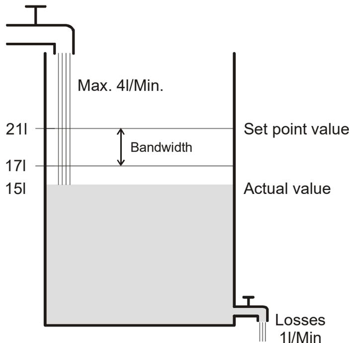
If the filling quantity is 15 l, there is a control deviation of  $21\text{ l} - 15\text{ l} = 6\text{ l}$
