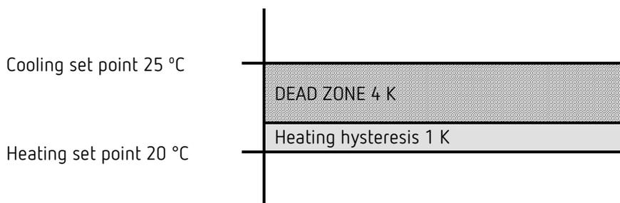
The dead zone (4 K) is increased by the value of the hysteresis (1K) and offsets the cooling set point value to 25 °C.
